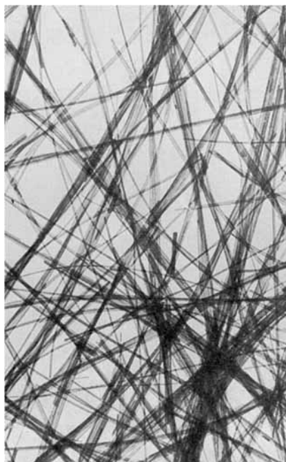
Fig. 14. Single fibrils of dispersed chrysotile asbestos. 12,500 \times .
