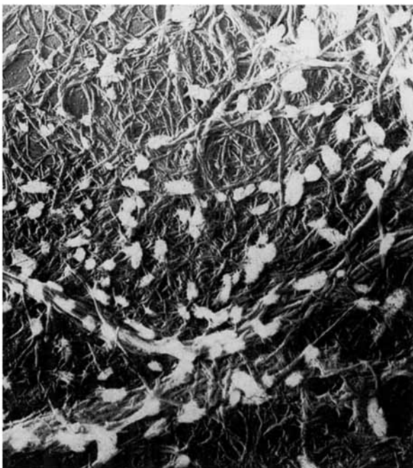
Fig. 3. Microfibrils of beaten wood pulp. 7,500 \times .
